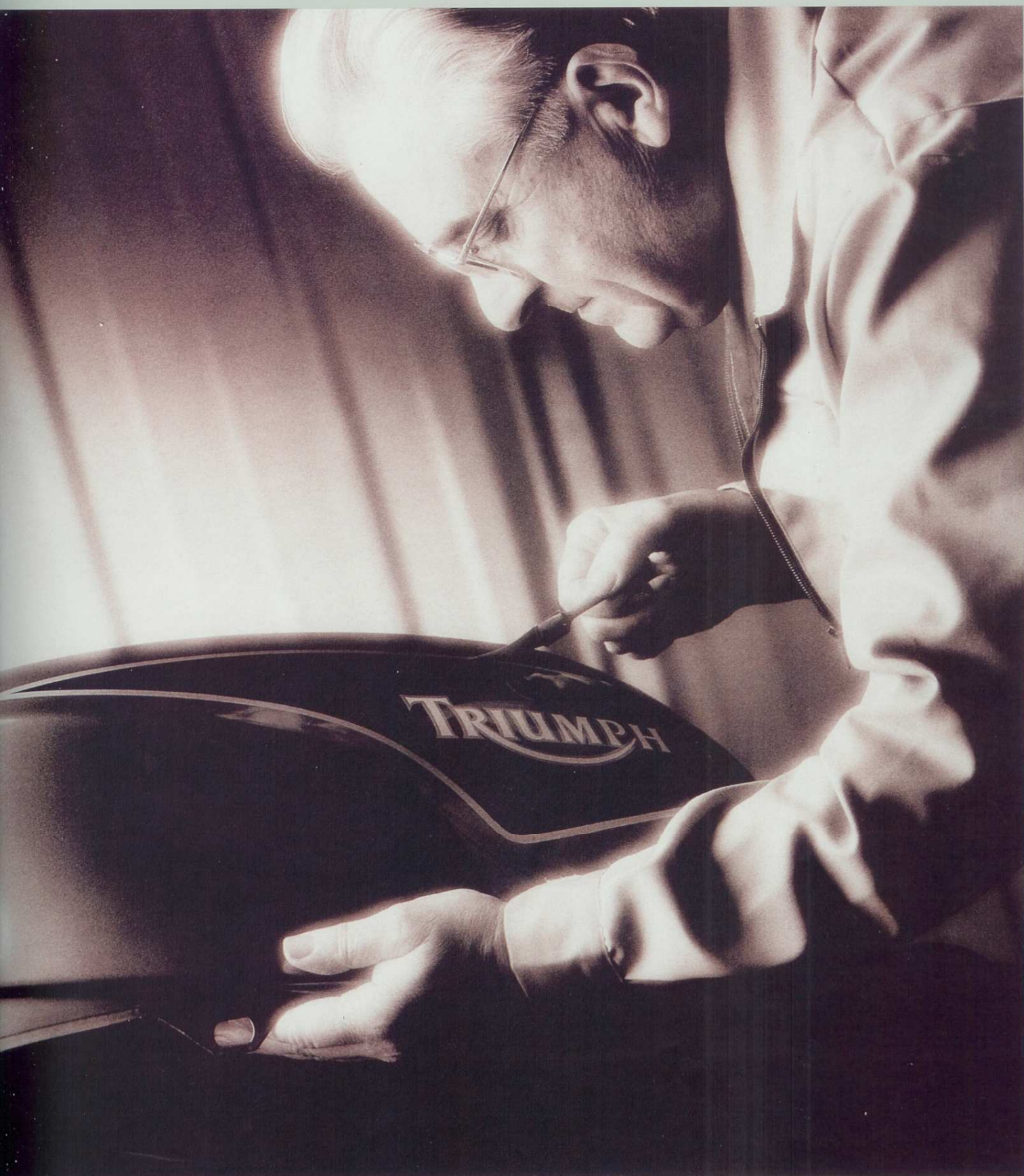
▲ Attention to detail at its best. Hand painting of coachlines on Triumph fuel tanks. A final lacquer coat enhances the finish. ◀ A detail check on paint prior to final assembly.
