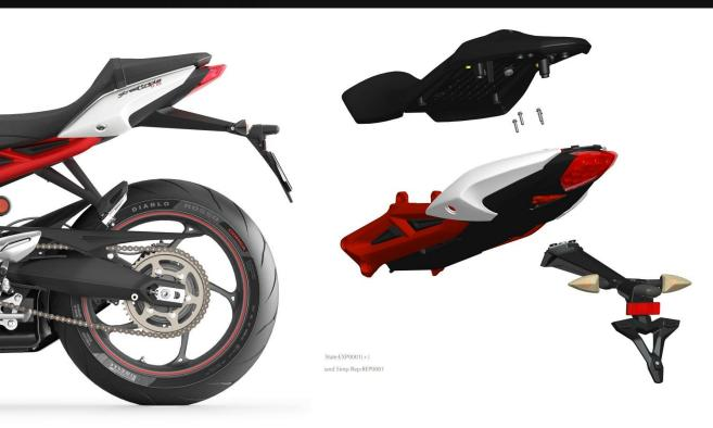
Rear end has been designed for easy removal of number plate hanger for occasional track use
