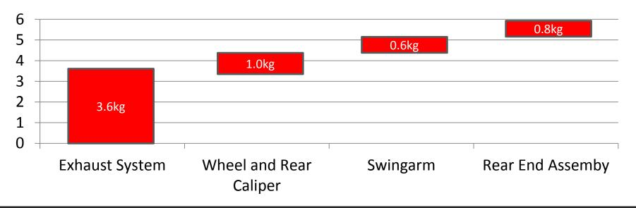
Most weight reduction has been from the rear end of the bike, contributing to a significant change in weight distribution
