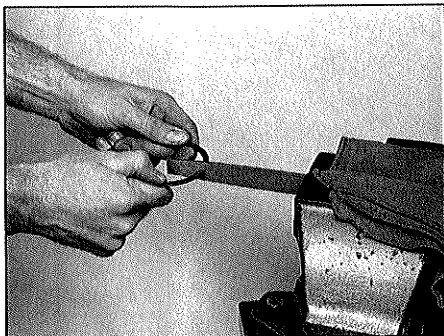
14.22 Ring end gap can be enlarged by clamping a file in a vice and filing
