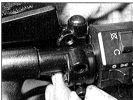
5.20a Fit the master cylinder and clamp to the handlebar making sure they are correctly aligned
