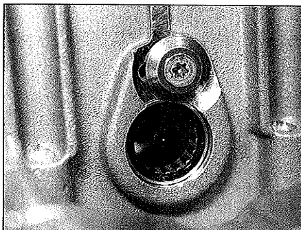
32.16b The needle roller bearing at the clutch end of the crankcase has a screw and washer on each side of the casing
