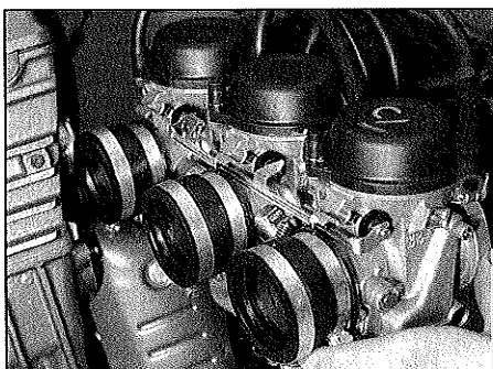
6.7b Ease the carburetors off the cylinder head with the rubber manifolds attached
