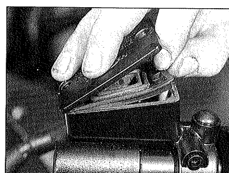
5.25 Make sure the diaphragm is properly seated, then fit the reservoir cover
