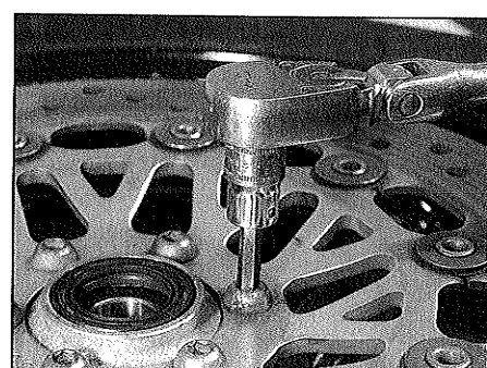
4.5 Unscrew the disc bolts a little at a time and in a criss-cross pattern to avoid distorting the disc
