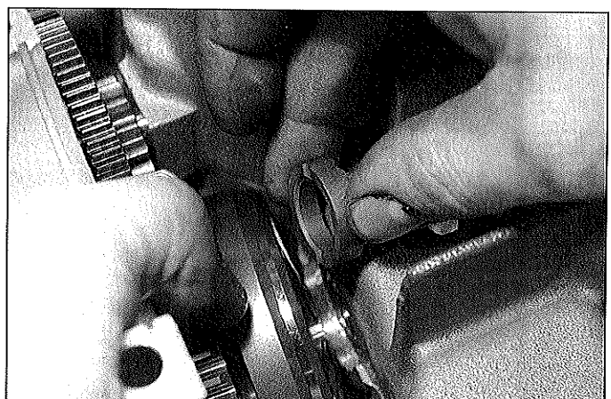
32.18 Tilt the starter clutch to one side to allow the spacer to be inserted
