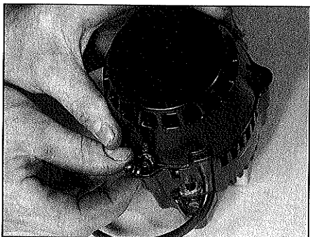
31.5 Unscrew the three nuts and detach the alternator end cover
