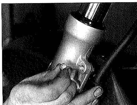
7.3a The mudguard is secured on each side by two bolts at the top ...
