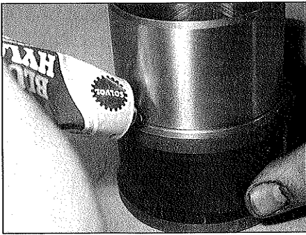
14.34a Apply a continuous bead of Blue Hylomar sealant to the liner seating . . .
