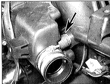
12.11 Locate airbox over rubber caps on subframe nuts (arrowed)
