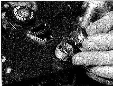
8.5 Unscrew the steering stem nut and remove the washer
