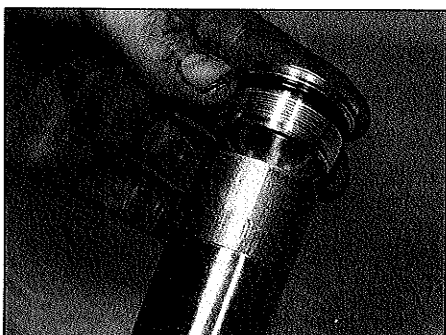
7.27 Fit a new O-ring to the top bolt, then install the bolt into the fork tube
