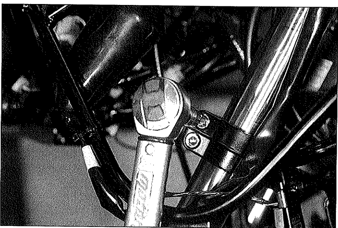
6.8b Tighten the bottom and top yoke pinch bolts to the specified torque setting
