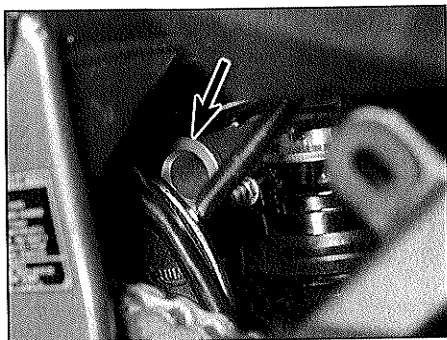
14.20b Install the spacer (arrowed) between the swingarm lugs before installing the spindle
