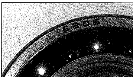
5.16 Typical bearing marking
