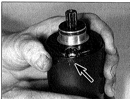
28.2b . . . and the end covers before disassembly (arrowed)
