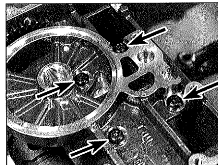
31.11 Release four screws (arrowed) to free the oil pump from the lower crankcase
