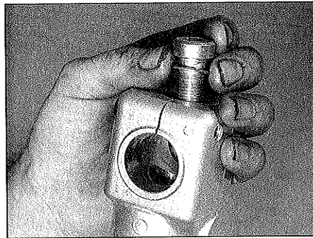
7.20a Fit a new sealing washer to the damper assembly bolt . . .
