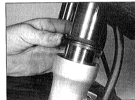
6.2 Inspect the area above the fork oil seal for oil leakage
