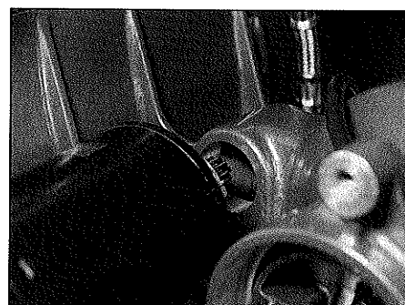
27.10 Slide the starter motor into position in the crankcase
