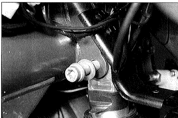
10.18 Install the shock absorber top mounting bolt
