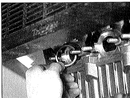
13.14 Fit a new gasket into each cylinder head port, with the flanged side inwards
