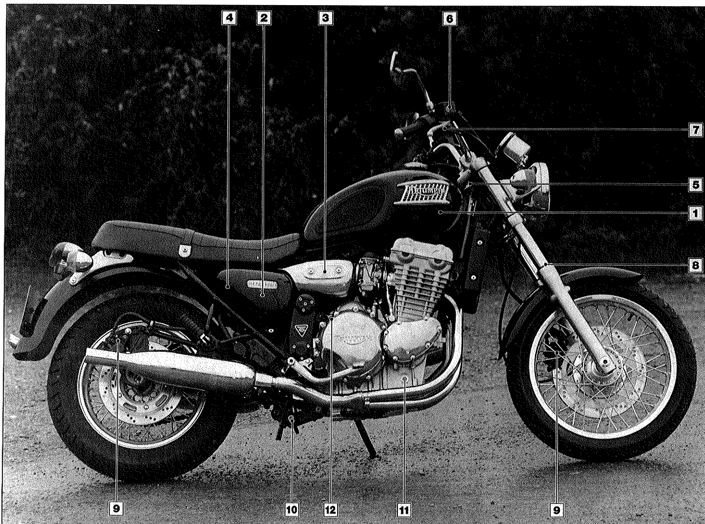
Component locations on right side (applies to Thunderbird, Thunderbird Sport, Adventurer and Legend TT models)
