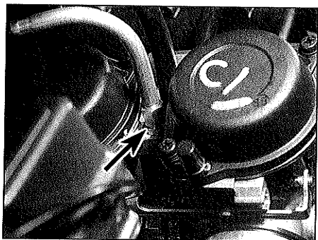
15.4b Lower adjuster is situated on carburettor (arrowed)
