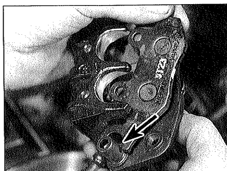
6.2g ... and remove the pads, noting how they fit against the lug (arrowed)
