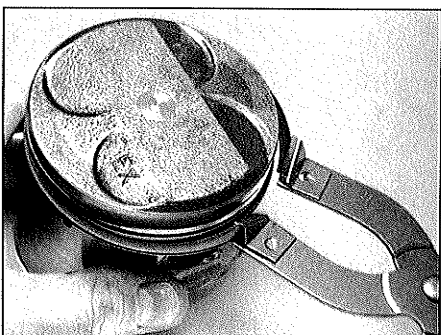
14.9 Compression rings can be removed with a ring removal and installation tool
