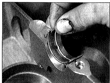
27.5 Slip the bearing shells to one side to remove them from their saddles
