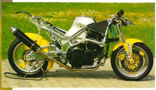
The Triumph triple engine was a prototype unit from the factory with Cosworth crankcases.
