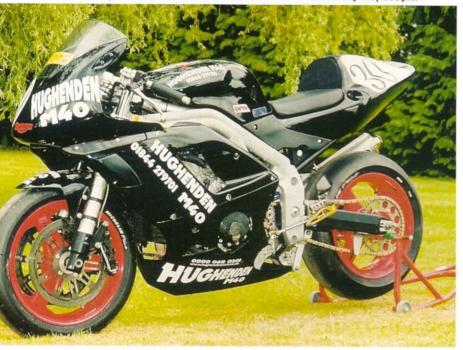
Rear suspension linkage arms have been replaced with longer machined items.
