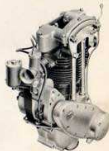
Engine of the "350" O.H.V. Model 3/2
