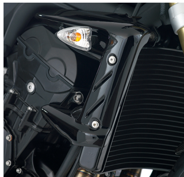
Colour Coded Radiator Cowl.jpg
