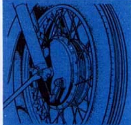
New Front Brake with 44% increase in area and more rigid drum.
