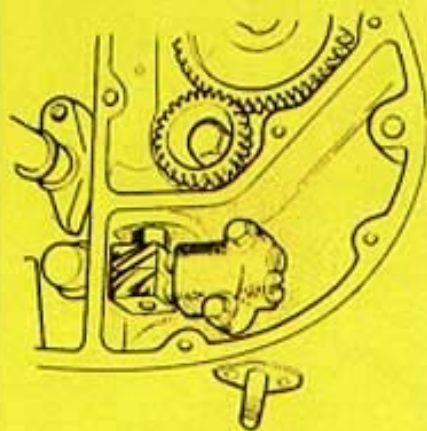
New Oil Pump of increased capacity on both feed and scavenge, with improved drive to plungers.
