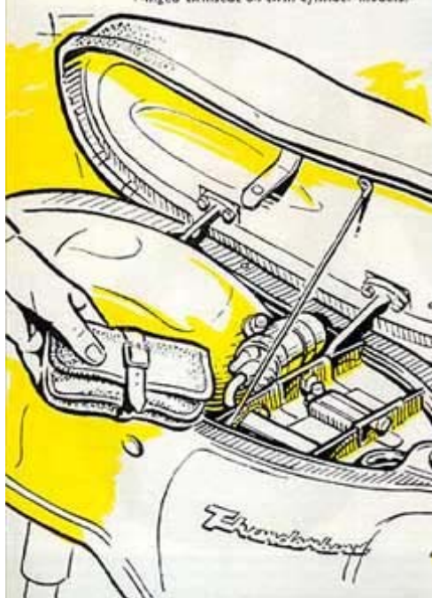
Hinged twinseat on twin cylinder models.
